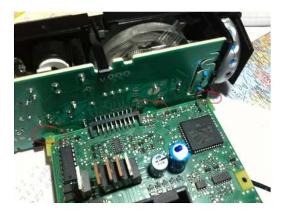
2. There's a small locating pin at the rear of the external housing that locates the circuit board. Fix - cut it off with a Stanley knife, as it pulls the rear circuit board away from the front board when you mount it in the housing. You could also apply some more epoxy here once you
